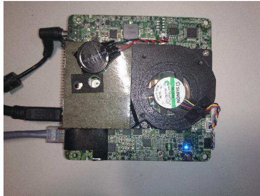
Fig. 7. 4"x4" NED prototype (~10.1x10.1 cm 2 )
